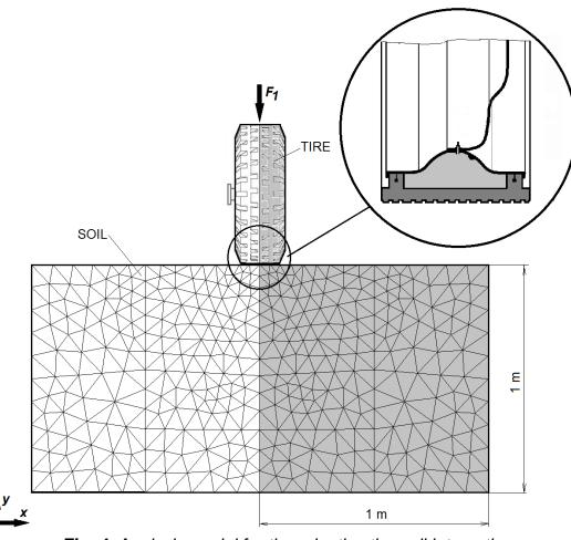
Fig. 4. Analysis model for the adaptive tire-soil interaction
