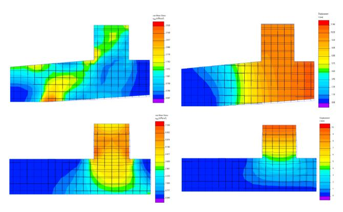
**Fig. 5.** Distribution of equivalent stresses in the adaptive tirein the contact area with the rolling track
